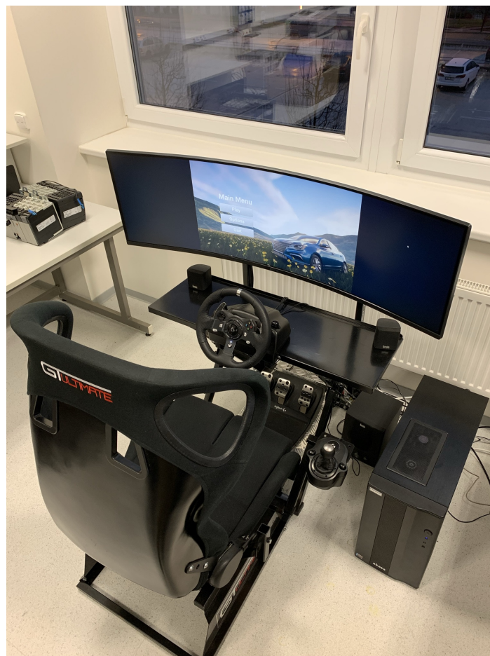
Figure 3. The hardware components of the Vehicle Driving Simulator.
