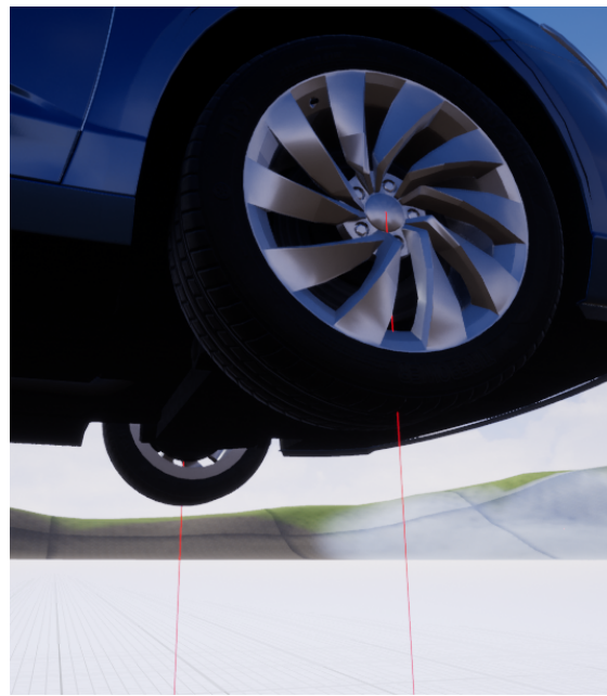
Figure 4. Wheels raycast curb detection.
