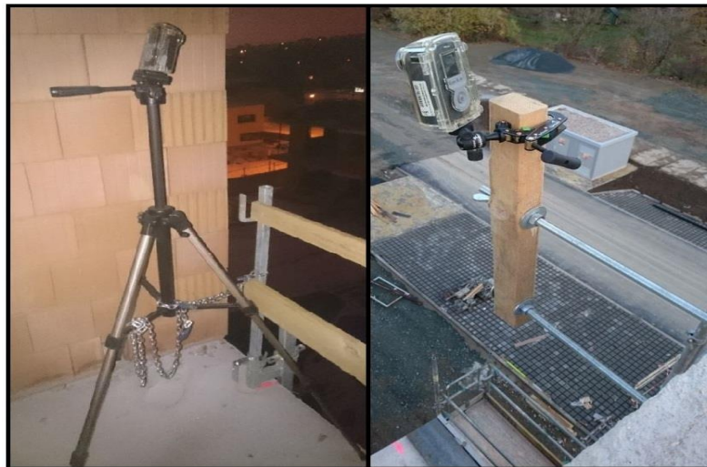
Figure 6. The device mounted on a tripod and a clamping bracket
