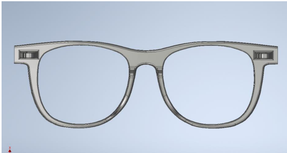
Obr. 29 Screenshot modelu obrouček z programu Solidworks 2020
