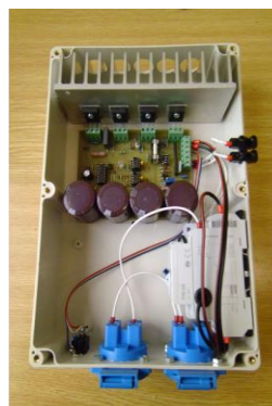
Obr. 2.12 MPPT Tracker + menič 2 kW [22]
