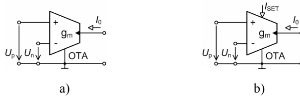
Fig. 1. Schematic symbol of OTA: a) with constant transconductance, b) with variable transconductance.
