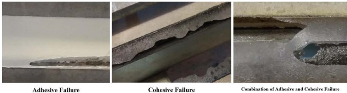
Fig. 3. Failure modes observed during testing.
