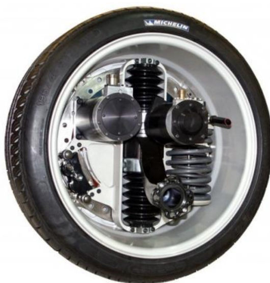
Obr. 50 Michelin Active wheel system [17]
