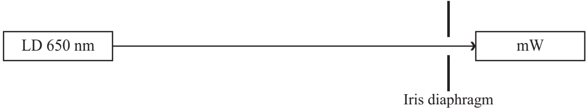
Fig. 4.2: Experimental setup of the geometrical attenuation measurement used to verify validity of Eq.(4.12) and Eq.(4.18). LD - laser diode with wavelength \lambda = 650 nm, mW - optical power meter. Distance z between the laser diode and Iris diaphragm was z = 0.2 m, where beam half-widths were w_x = 1.72 mm and w_y = 0.48 mm and axial optical intensity I(0, 0, z) = 2583 W/m 2 . Diaphragm diameter 2r_{\text{RXA}} was calibrated and adjustable in range 2r_{\text{RXA}} \in < 0.5; 5 > mm with 0.5 mm step.
