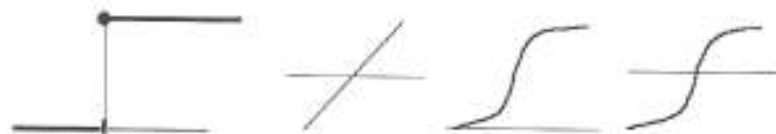
Fig. 2 - Activation functions hardlim, purelim, logsig, tansig; source: (7)
