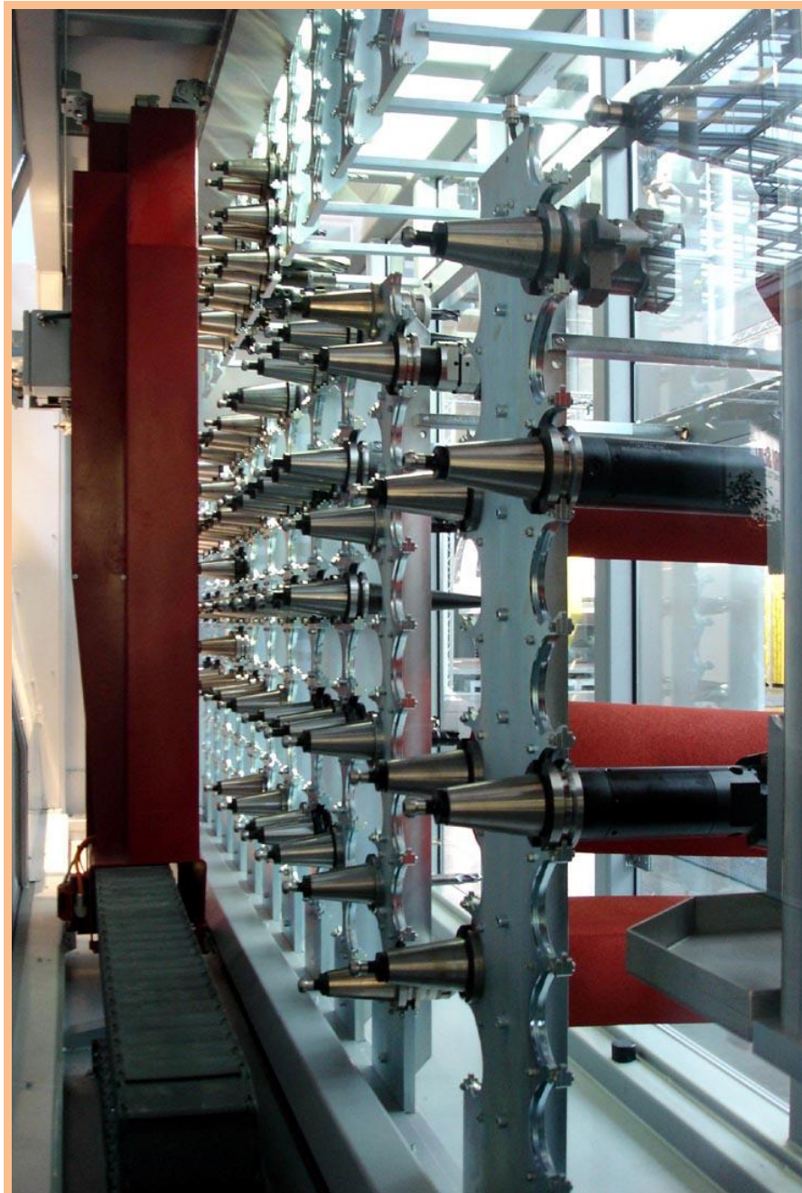
Obr. 39 Matrix Tool Magazine od firmy Toyoda [5]
