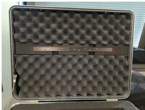
Fig. 23 T-SCAN Hawk 2 with HyperScale scale calibration bar
