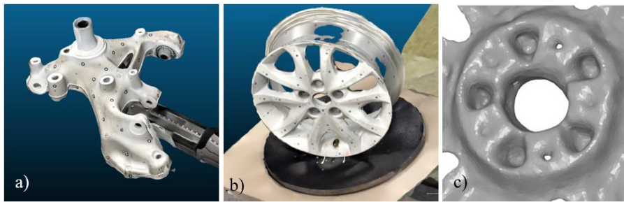
Fig. 29 iPhone LiDAR mesh: (a) steering knuckle with texture; (b) car wheel with texture; (c) car wheel's hub mesh
