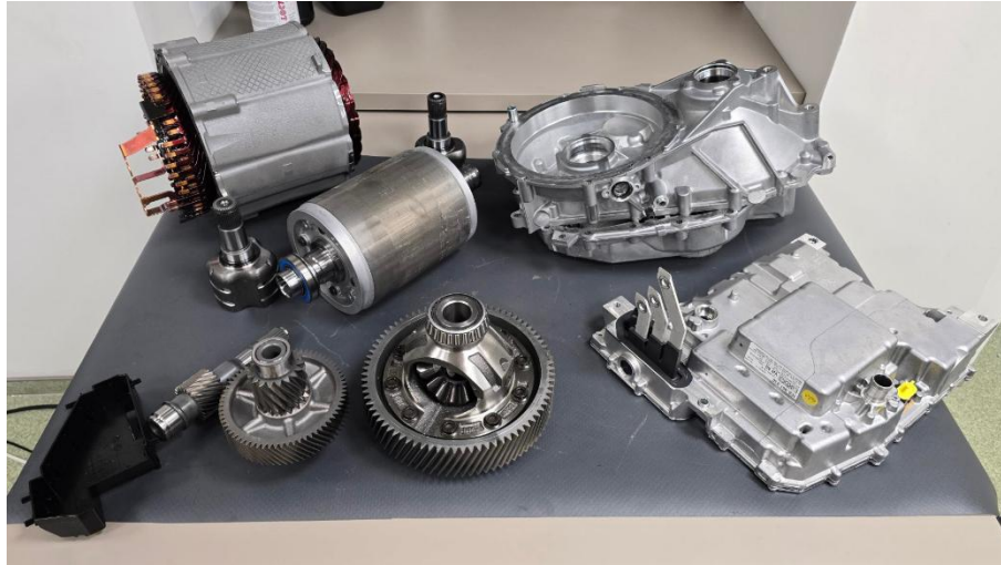
Fig. 42 Components of the 1-speed transmission unit 0MH (Audi Q4 e-tron)
