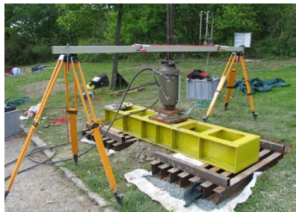
Fig. 2. (a) the investigation test setting up; (b) bridge for the independent measurement of the tendon displacement.
