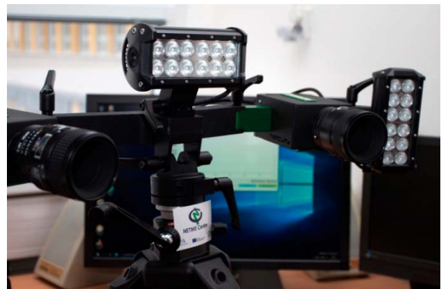
Fig. 5. Mercury RT optical device for measuring deformities.
