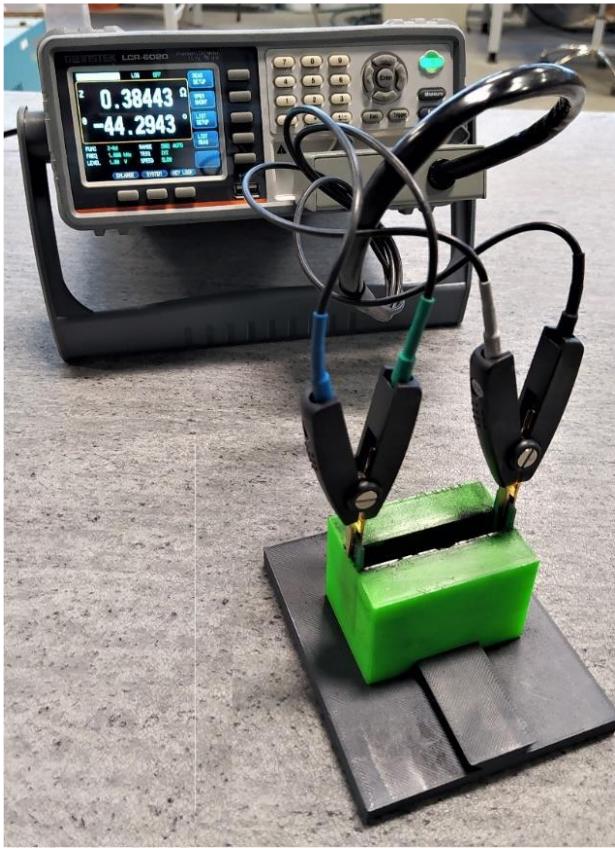
Figure 1. Measuring device GW Instek LCR-6020.
