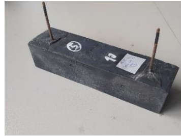
Figure 2. Composite test specimen for impedance measurement.
