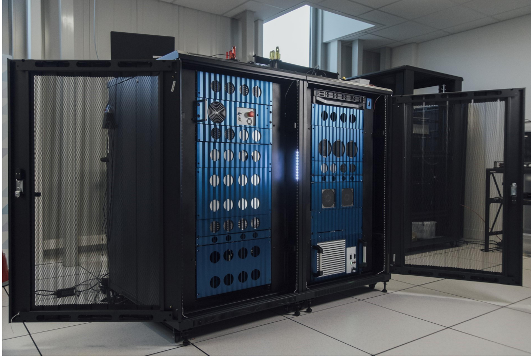
Figure 2.3: The Lucy quantum computer, a photonic system developed by Quandela and hosted at the TGCC (CEA), France. Source: https://www.eurohpc-ju.europa.eu/eurohpc-quantum-computers/our-quantum-computers_en . Author: Agence Oblique/-Cyril Marcilhacy
