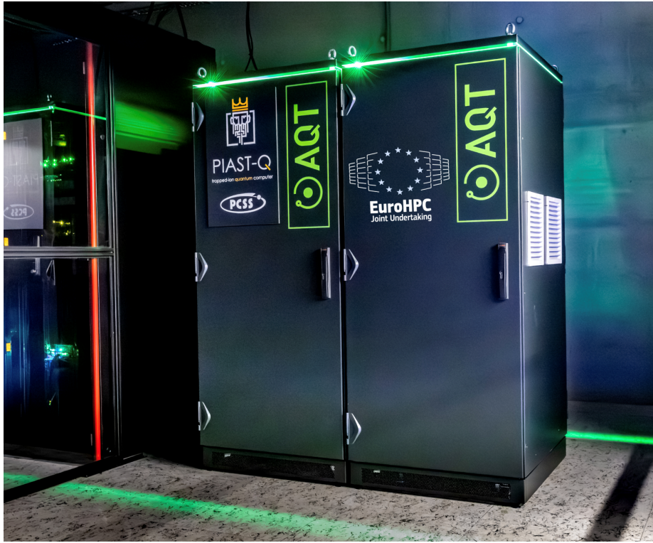
Figure 2.4: The PIAST-Q quantum computer, a trapped-ion system developed by AQT and hosted at the Poznań Supercomputing and Networking Center (PSNC), Poland. Source: https://www.eurohpc-ju.europa.eu/eurohpc-quantum-computers/our-quantum-computers_en . Author: PSCN
