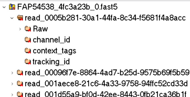
Fig. 1. Hierarchy scheme of a FAST5 file containing 4 reads, the first read showing the groups ‘Raw’, ‘channel_id’, ‘context_tags’ and ‘tracking_id’
