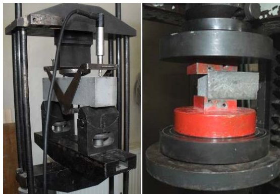
Fig. 2: Arrangement of three-point bending fracture test (left) and determination of an informative value of compressive strength
