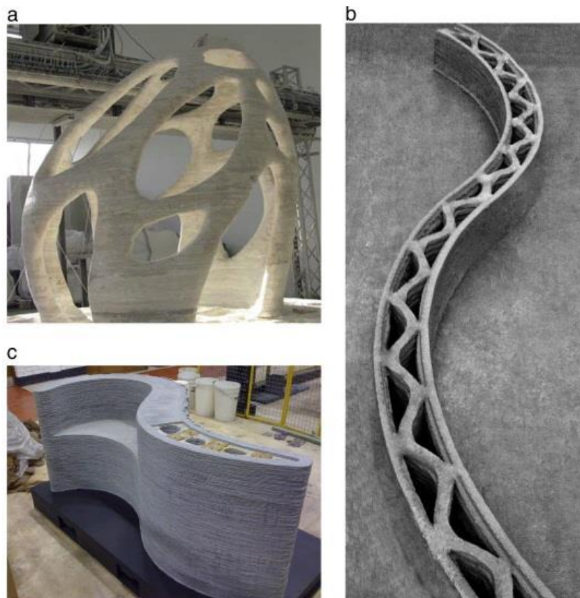
Obr. 22 D-shape, contour crafting, concrete printing [17]
