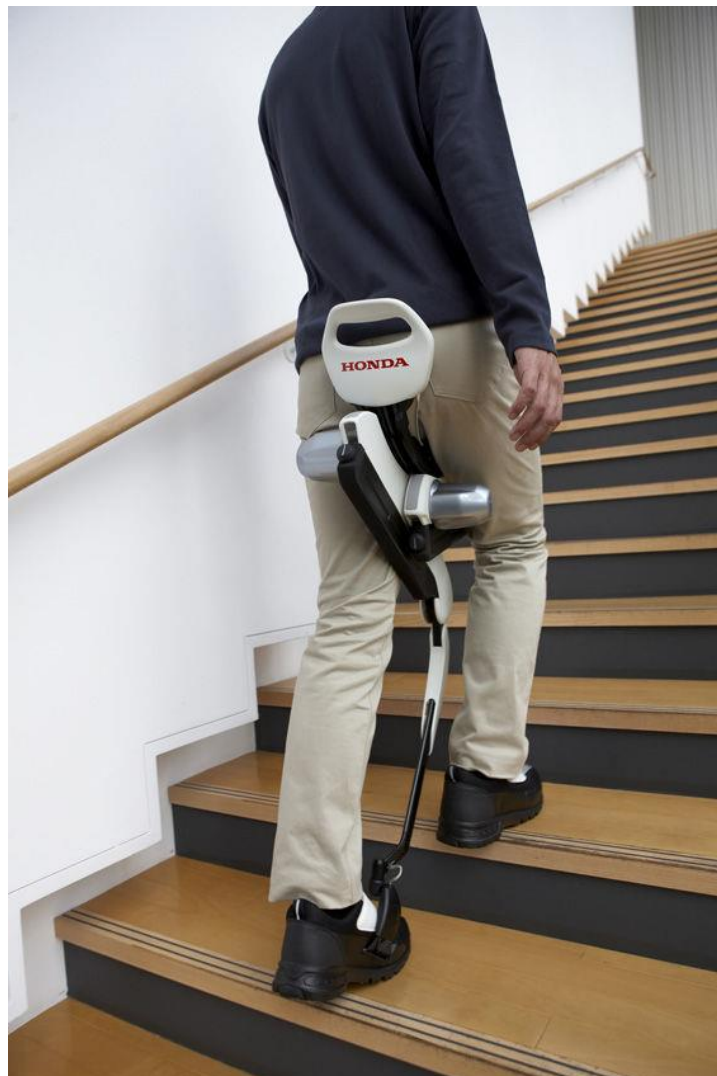
Obr. 4.4 Pouiti ortezy Walking Assist Device with Bodyweight Support Assist pri chuze do schodu [12]
