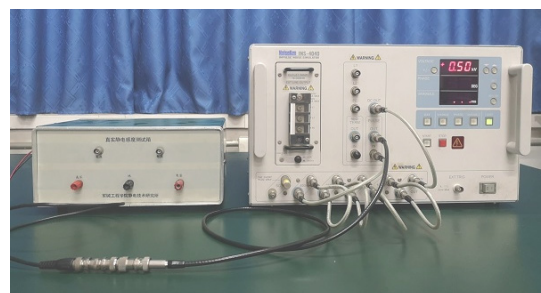
Fig. 7. The ignition excitation test system of the electric explosive device as impacted by the electromagnetic pulse.
