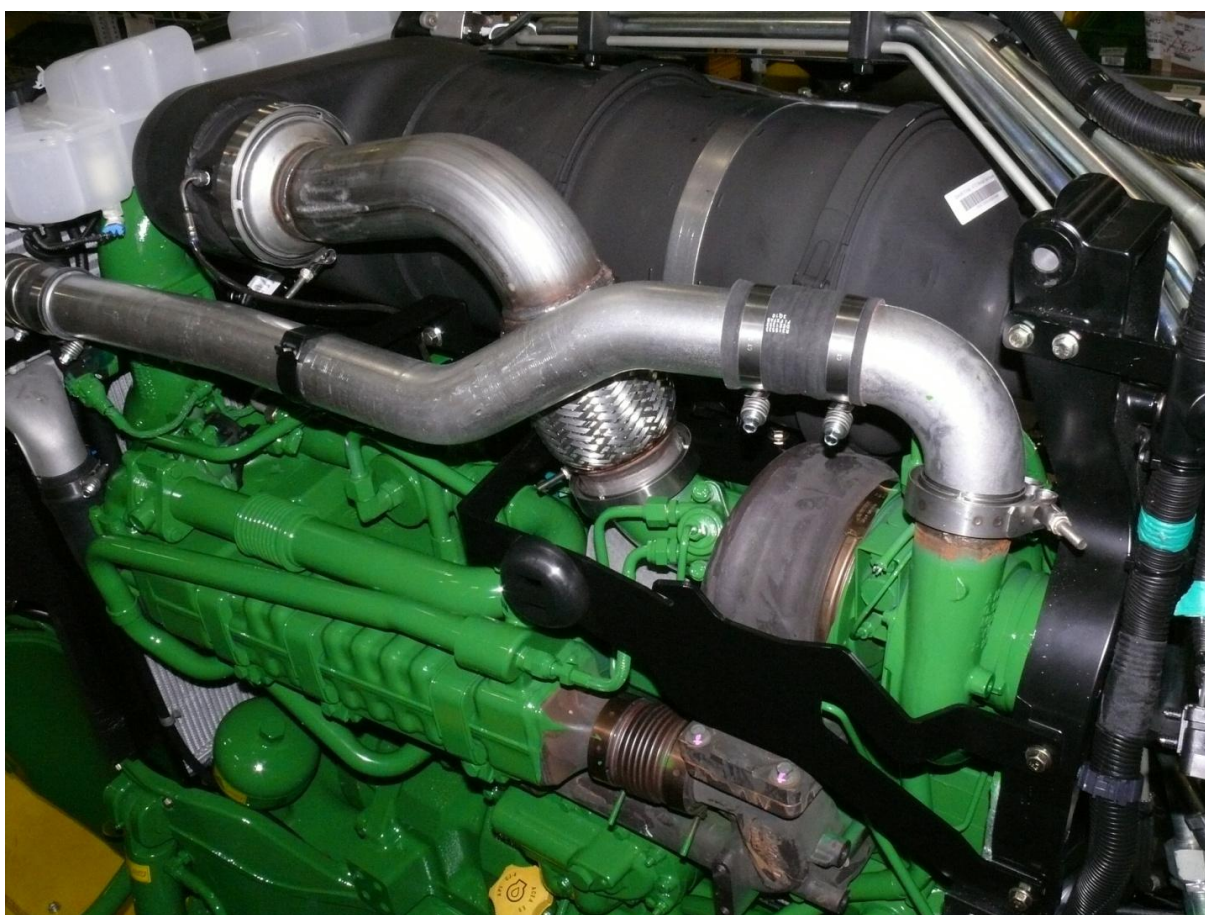
Obr. 4.2.5. DOC a DPF filtr motoru John Deere [15]
