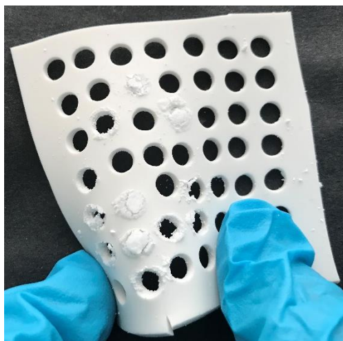
Figure 18: The fragile and disintegrated LYSSTAPH-S lysostaphin-loaded CPC samples after curing in the incubator.
