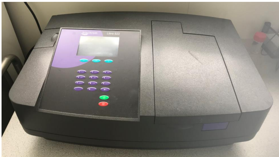
Figure 20: UV-VIS spectrophotometer Biochrom Libra S22 used for the release measurement.
