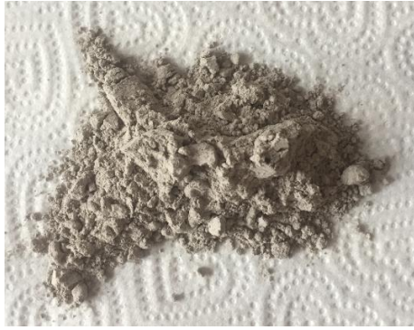
Fig. 6. Filler FHW1 (quartz powder, FBC, EP).
