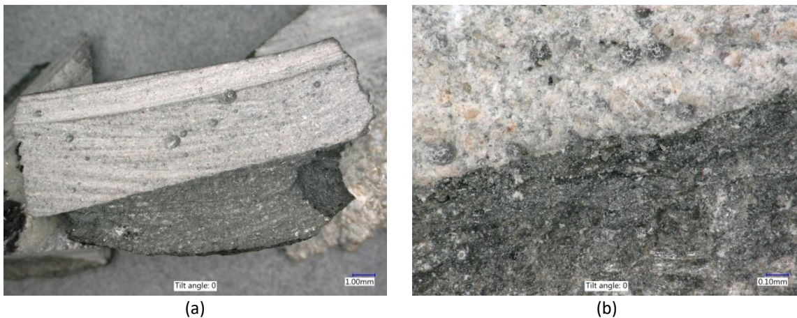
(a) (b) 9 Fig. 25. The connection of the HRG-D grout to the cat basalt element: (a) magnification 6.4x; 10 (b) magnification 16x.
