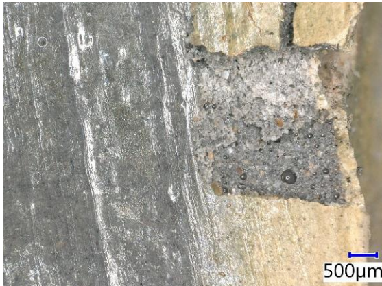
Fig. 31. HRG-D grout – transverse view of grout interface (REF/HCl) at the indentation site.
