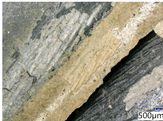
Fig. 30. Separation of ERG-D grout from cast basalt element after exposure to HCl.
