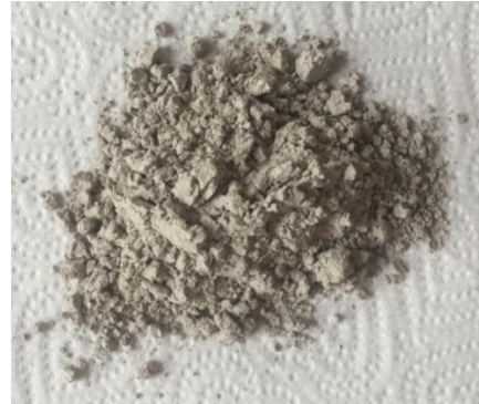
Fig. 7. Filler FHW2 (quartz powder, FBC, CBD).
