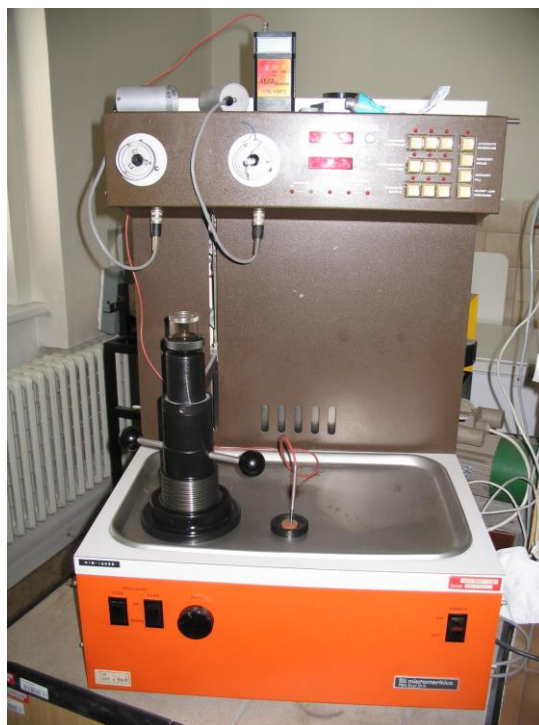
Obr. 15 Porozimetr Micromeritics PoreSizer 9310
