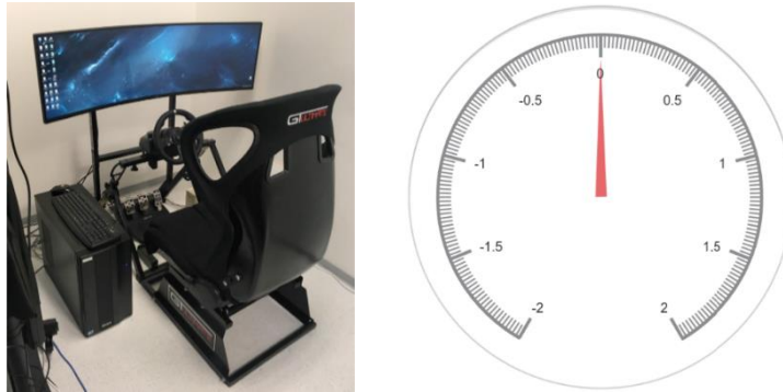
Figure 2: Vehicle driving simulator [3] and regulation error indicator
