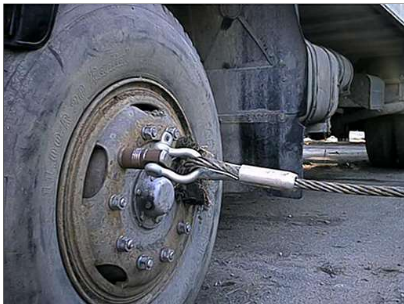
Obr. 4 - Detail úchytu – matice s okem Fig. 4 - Detail of hitch – female screw with loop
