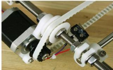
Figure 5. Mechanical endstops. Adopted from Evans (2012) “Practical 3D Printers”
