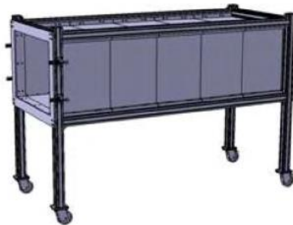
FIGURE 15: TEST SECTION, 5 GLASS WINDOWS [10]
