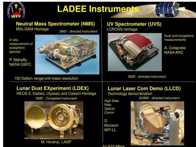
Figure 1.8 LADEE science and technology payload instruments[42].
