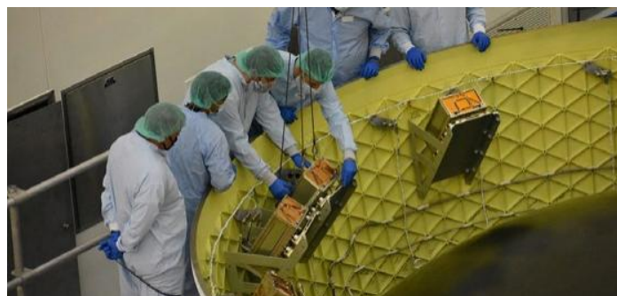
Figure 1.2 The Artemis I Orion stage adapter with mounting brackets for secondary[17].
