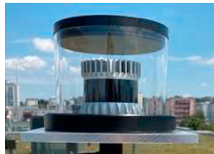
Fig. 3. Ouster OS1 with 64 lines in vertical direction and the transparent cover
