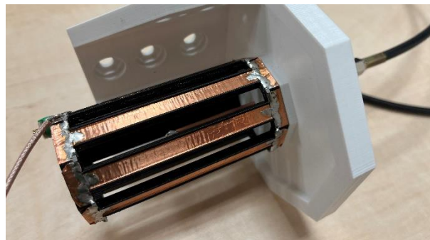
Figure 5: Measurement setup (the probe is located in the centre of the resonator)
