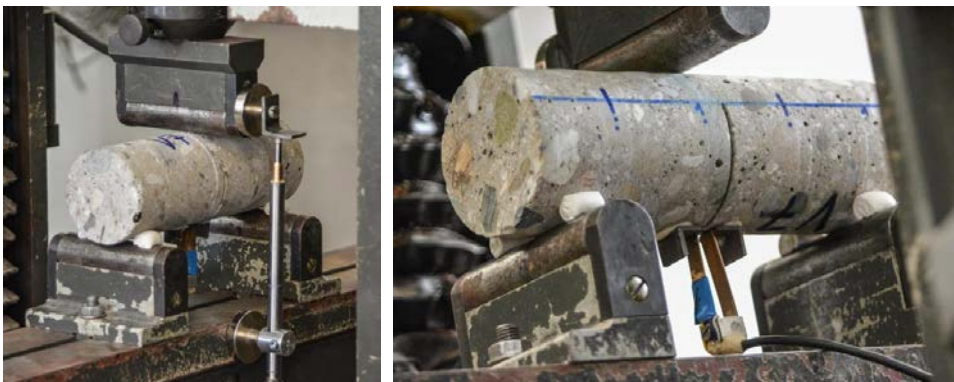
Fig. 3. Three-point bending fracture test of specimen V7 – details of measurement of displacement d (left) and CMOD .
