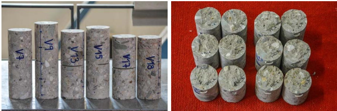
Fig. 1. Specimens before (left) and after fracture test.
