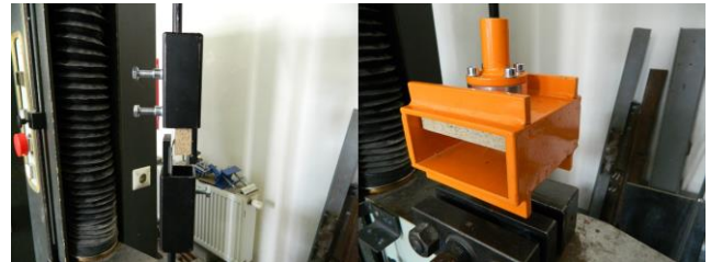
Figure 2. Testing of specimens in testing equipment (shear – left, bonding – right)
