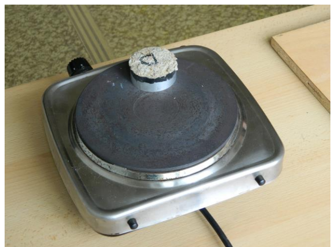
Figure 3. Heating of a specimen on a hot plate
