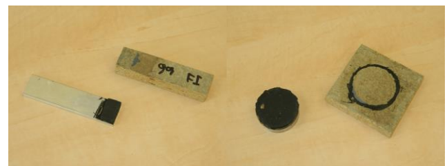
Figure 4. Test Test specimen after testing (shear – left, bonding – right) – HQ Bond
