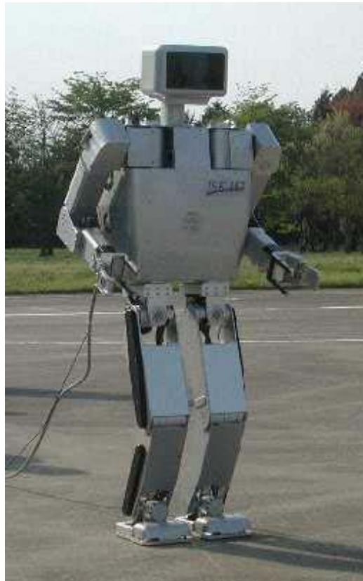
Picture no.3 - Isamu stands 1,346 mm tall, weighs 54,9 kg, and walks at over 1,6 km per hour. Not only that, Isamu climbs up and down stairs, carries 1,8 kg objects in its hand-like grippers, and even recognizes human faces via its dual-camera stereo vision system. [15]
