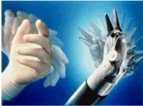
Picture no.7 - How the hand of DaVinci surgeon is following the motion of a human surgeon. It is very accurate. [16]
