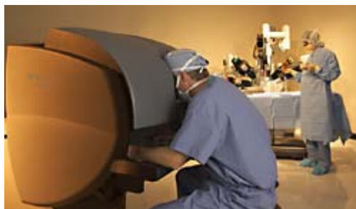
Picture no.5 - How DaVinci works - the surgeon sits from a distance and guides DaVinci to do the precise surgery. [16]
