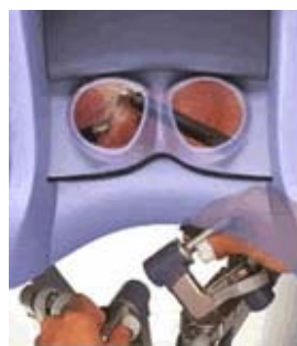
Picture no.6 - We can see where is the surgeon looking into, the daVinci surgeon has two cameras that show the inside of the patient and the human surgeon is using his hands to guide the hands of the daVinci surgeon to do the precise work. [16]
