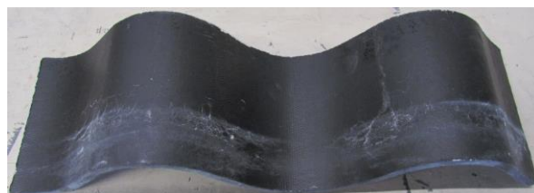
Figure 3. Sample of fibre-cement profiled sheet after 100 cycles of freeze-thaw.
