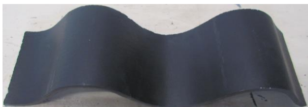
Figure 2. Sample of fibre-cement profiled sheet before freeze-thaw test.
