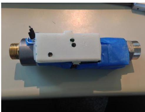
Figure 3: The final prototype of the sensor casing mounted with control electronics
