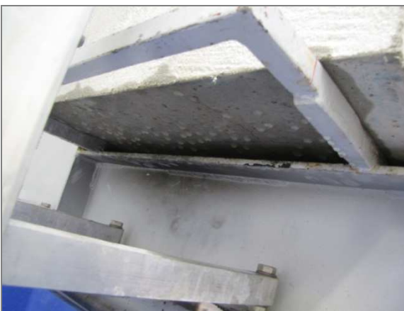
5. Water vaporization and condensation on the bottom surface of specimen (47 min)
