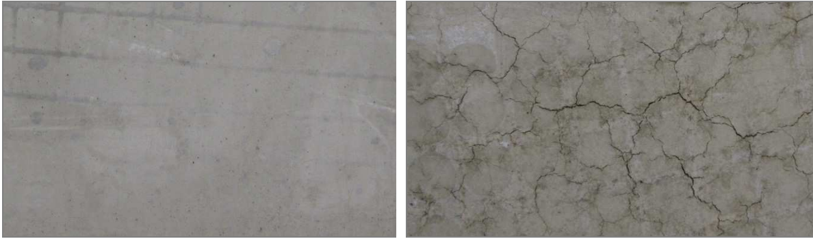
Figure 10-17: Left: Detail of exposed surface before fire test; Right: Cool down specimen after fire test
