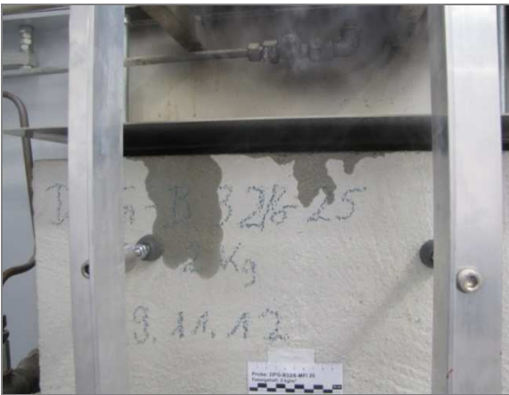
3. Water vaporization and condensation on the top surface of specimen (26 min)
