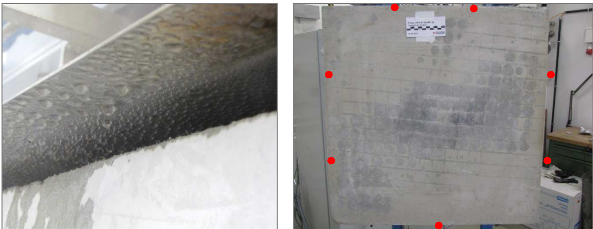
Figure 10-19: Left: Water vaporization and intensive condensation on the top surface of specimen (00:47); Right: Location of crack formation occurred in first 5 minutes (DFG B15/6 - MFI25 - 2 kg/m 3 ) (by author)
