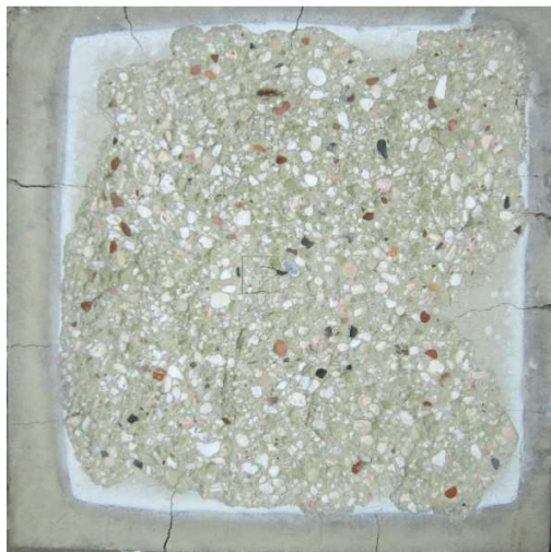
Figure 10-21: DFG-R- without fibers – spalling depth up to 20 mm
