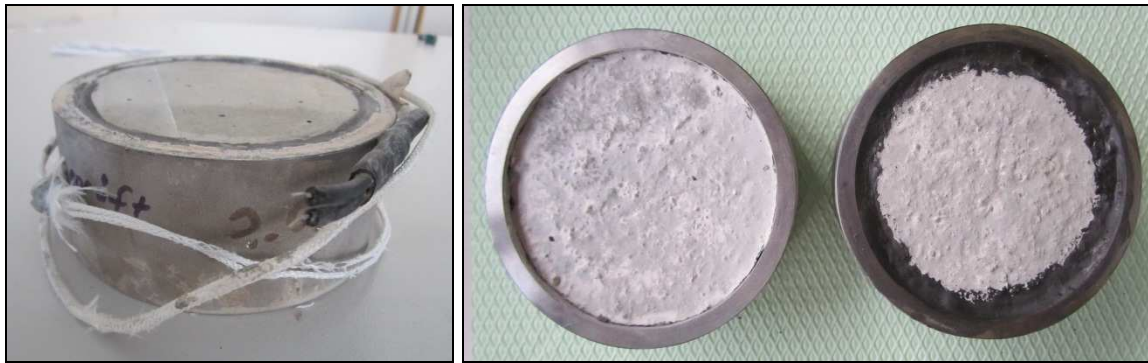
Figure 11-1: Concrete samples placed in steel rings (left: specimen with thermocouple)
