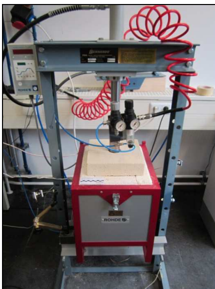
Figure 11-13: Electric furnace ROHDE in the frame (by author)
