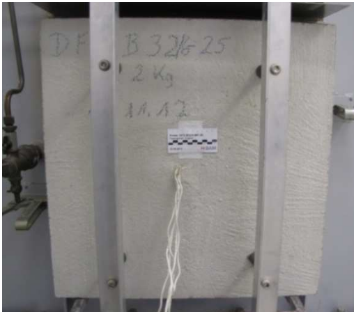
1. Before fire test (00:00)
