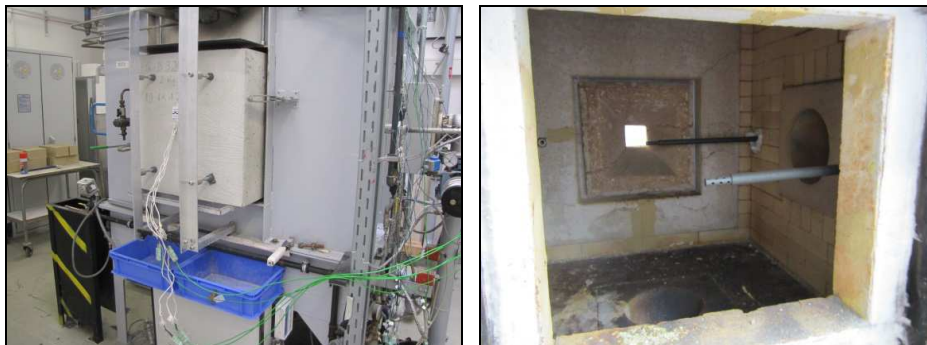
Figure 10-13: Testing 1m 3 furnace (by author)
