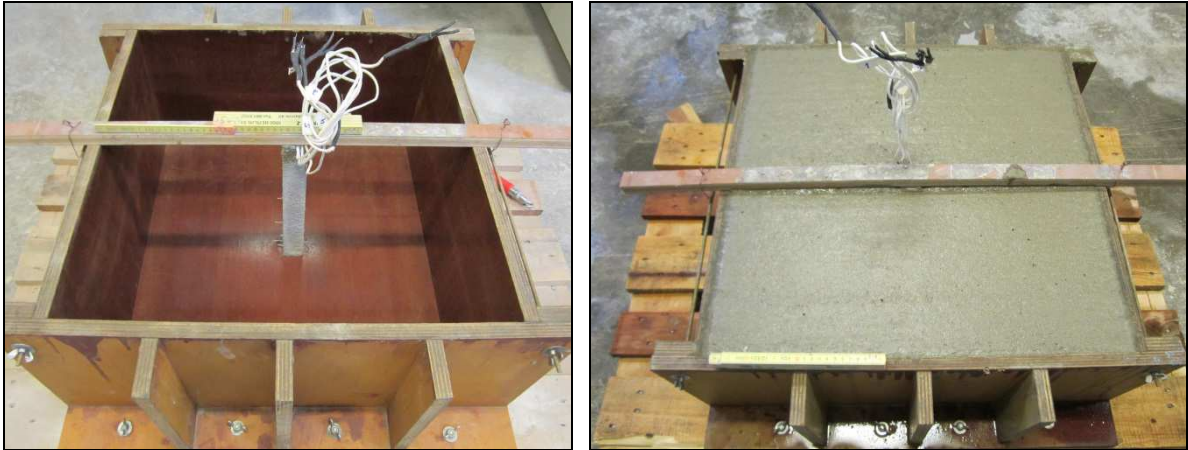
Figure 10-3: from the left: 1) pre-prepared mould with positioned prism with thermocouples, 2) full-filled mould (by author)
