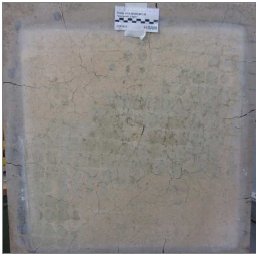
Figure 10-22: DFG-B15/6 - MFI25-2 kg/m 3 - spalling volume 0%, only cracks and deformation
