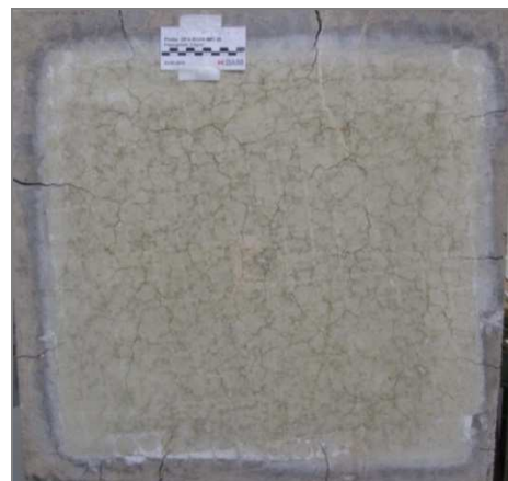
6. Cool down specimen after fire test
