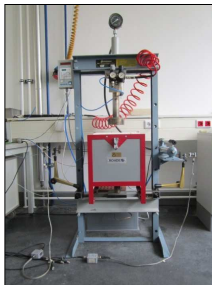
Figure 11-13: Electric furnace ROHDE in the frame (by author)
