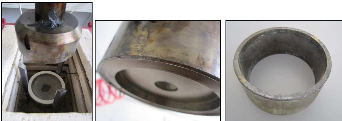
Figure 11-15: from left: sample holder, pressure plunger and sample ring (by author)
