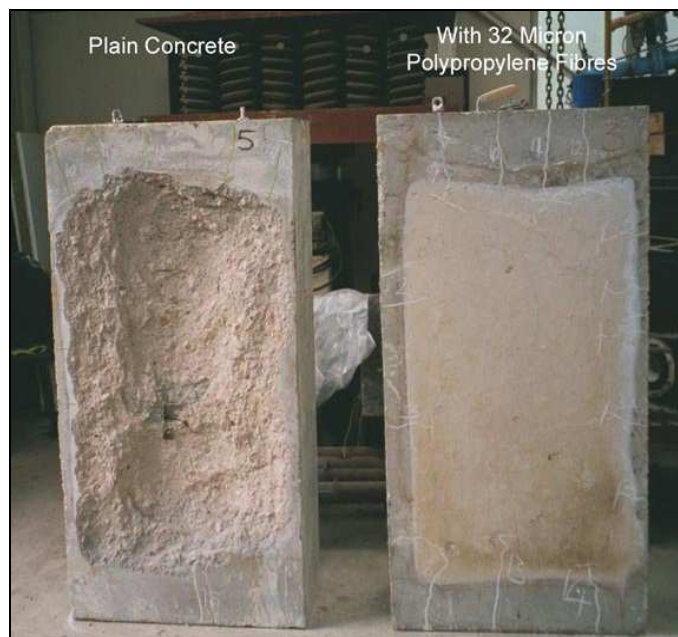
Figure 2-1: Spalled surface of concrete without PP fibres and with PP fibres [16]
