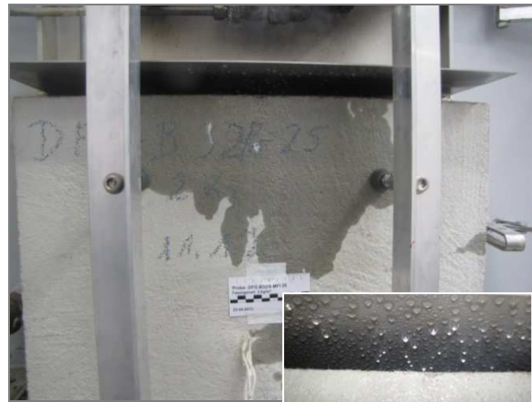
4. Water vaporization and condensation on the top surface of specimen (45 min)
