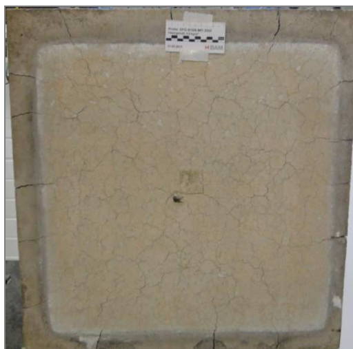
Figure 10-22: DFG-B15/6 - MFI25-2 kg/m 3 - spalling volume 0%, only cracks and deformation
