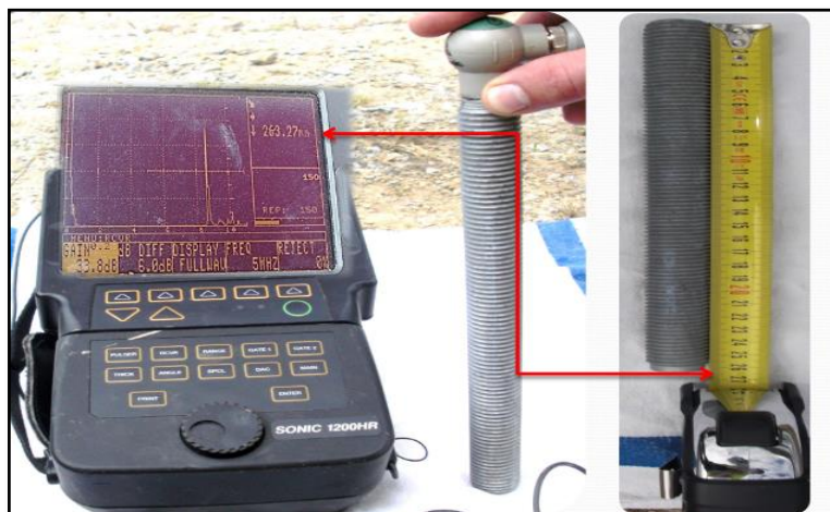
Figure 1. Setting and calibrating the US of the instrument.
