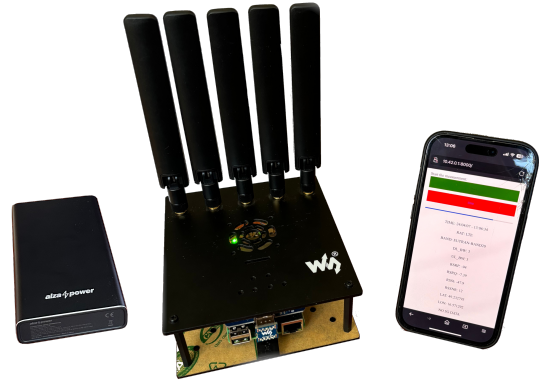
Fig. 1. Measurement setup: (left) battery pack, (middle) measurement device, (right) equipment to visualize data.
