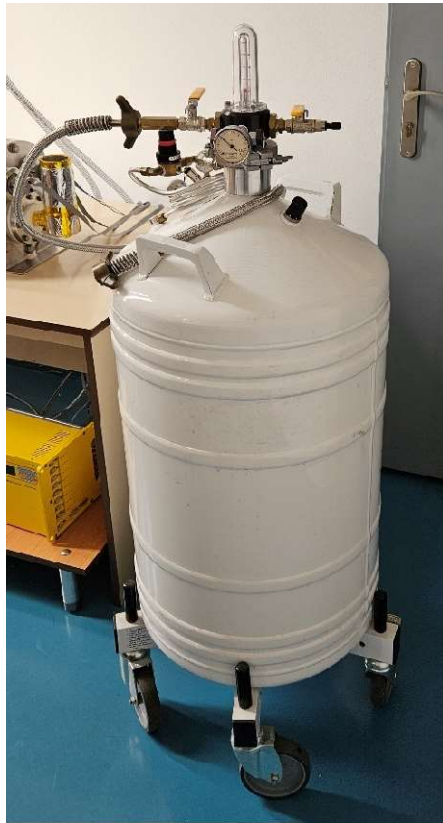
Figure 12.10 Liquid nitrogen tank
