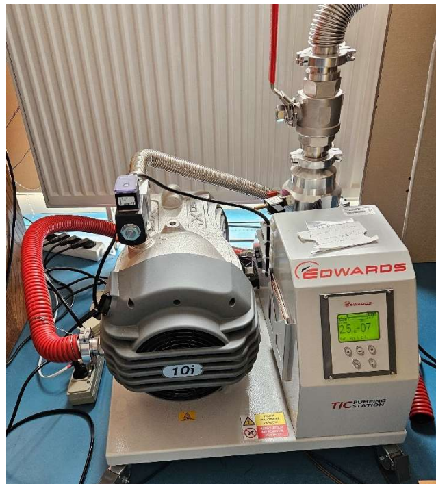
Figure 12.4 Turbo-pumping station with TIC
