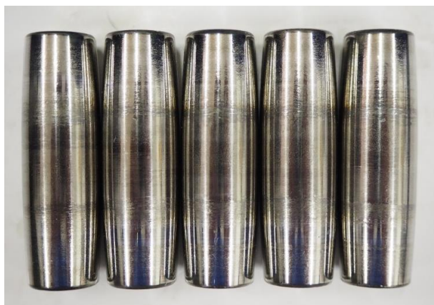
Figure 51. Number of the rolling elements of the toroidal bearing after the test.
