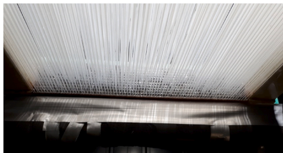
Fig. 1. Typical configuration of heat transfer surface from polymeric hollow fibers for gas-liquid HX.
