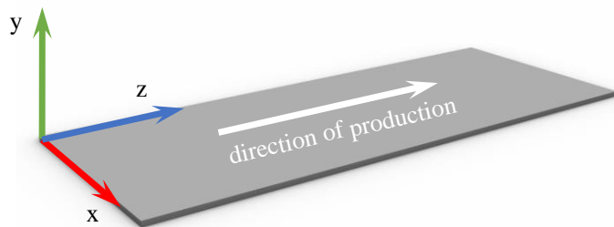
Figure 2. Scheme of loading directions with regard to the direction of production of cement fiber boards produced by the Hatschek method
