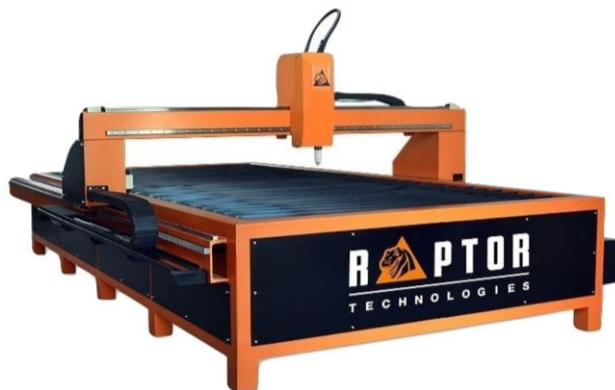
Obr. 2) CNC Router Raptor Beast 30/15 [3]
