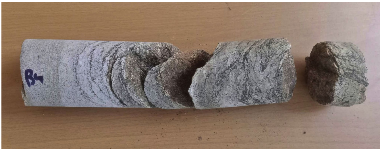
Fig. 2 Example of an extracted migmatite core section with prevailing discontinuities limiting the possible length of a prepared cylindrical specimen
