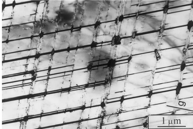
Fig. 10 Nucleation of \alpha' martensite in the intersection of \epsilon martensite plates after cyclic loading with total strain amplitude 1.6 \times 10^{-2} [5].
