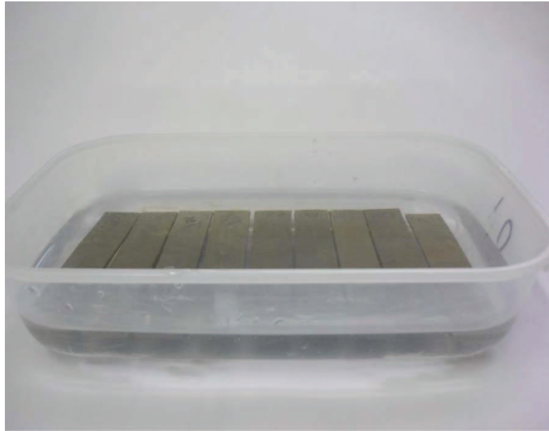
Fig. 14 MDF specimens exposed to distilled water
