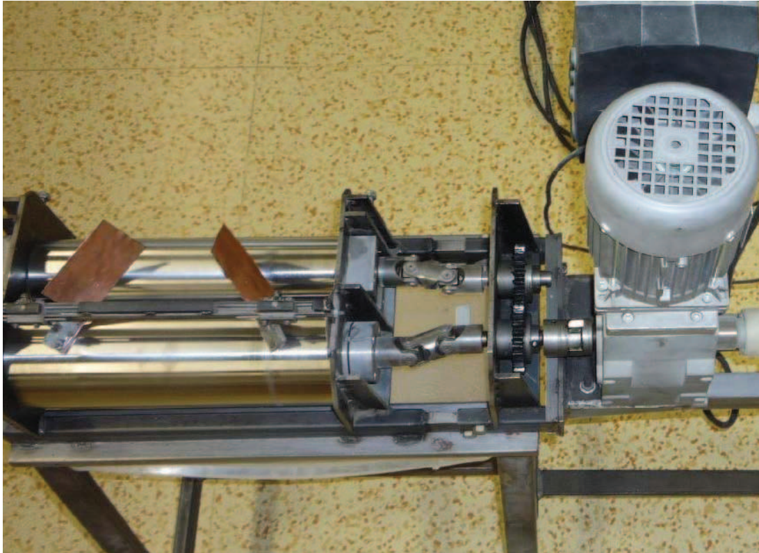
Fig. 12 Two-roll mill for high-shear mixing
