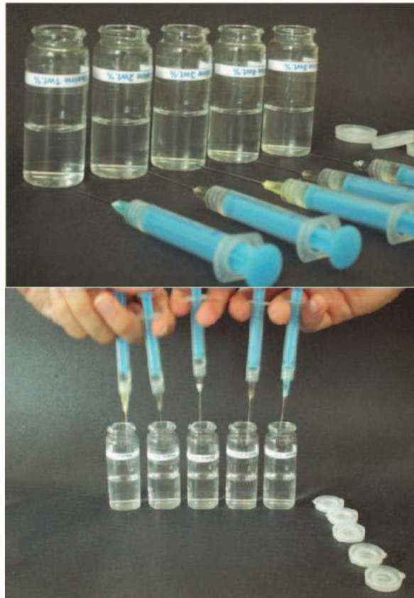
Fig. 11 Gel point determination by tilted test tube method
