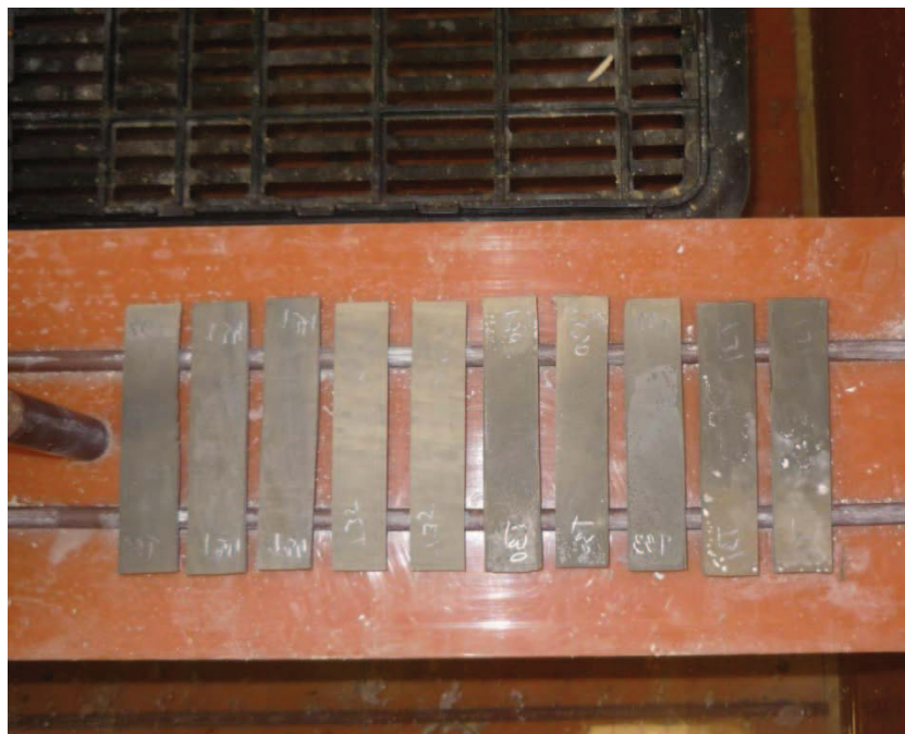
Fig. 13 MDF specimens exposed to humidity
