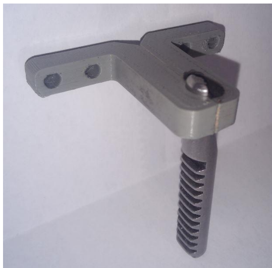
Model čelistí uchopovače 1
