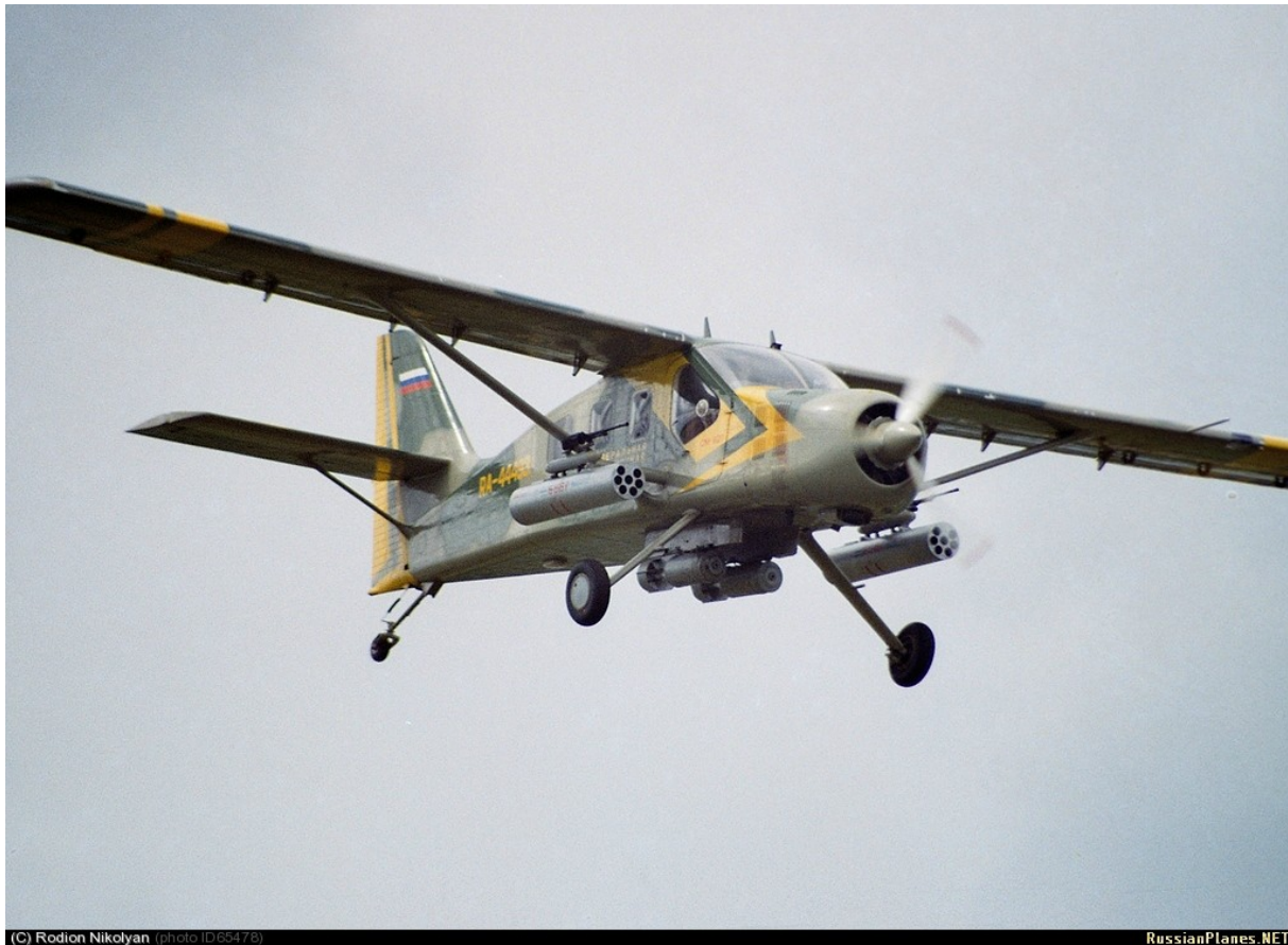
Figure 1.1: Military version of SM-92 with radial engine [29]
