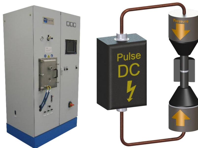
Fig. 18 FCT Spark-Plasma Sintering furnace and schema of the principle [26].
