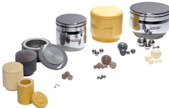
Fig. 13 Milling bowls and elements with different volumes and materials.
