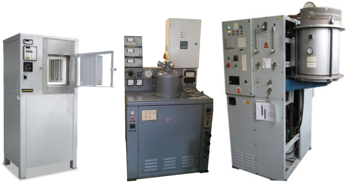
Fig. 17 Conventional furnace Nabertherm (left), Vacuum furnace Degussa (middle) and hydrogen furnace Novex (right).
